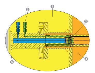
Figure 2 The GPro 500 Interface between Zone 0 and Zone 1
